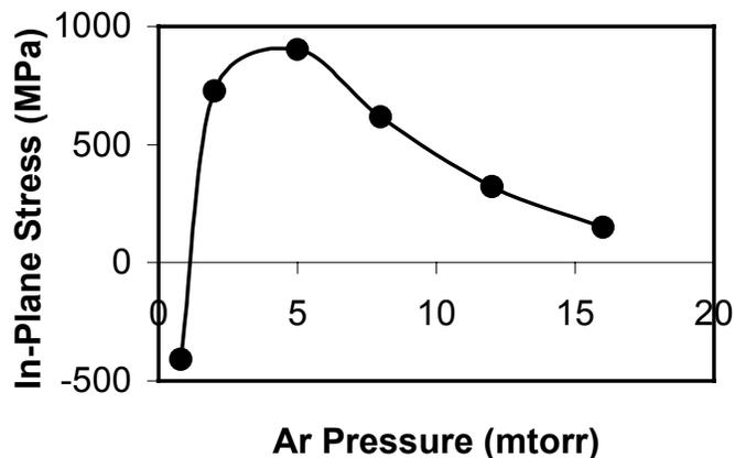
Fig.1 In-plane stresses vs. Ar pressure. Negative values represent compressive stress whereas positive values represent tensile stress.
