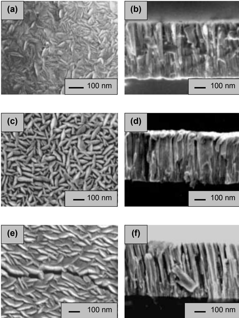
Fig. 3. SEM planar and cross-sectional views for Mo films sputtered (a and b) at 0.8 mtorr, (c and d) at 5 mtorr, and (e and f) at 8 mtorr.
