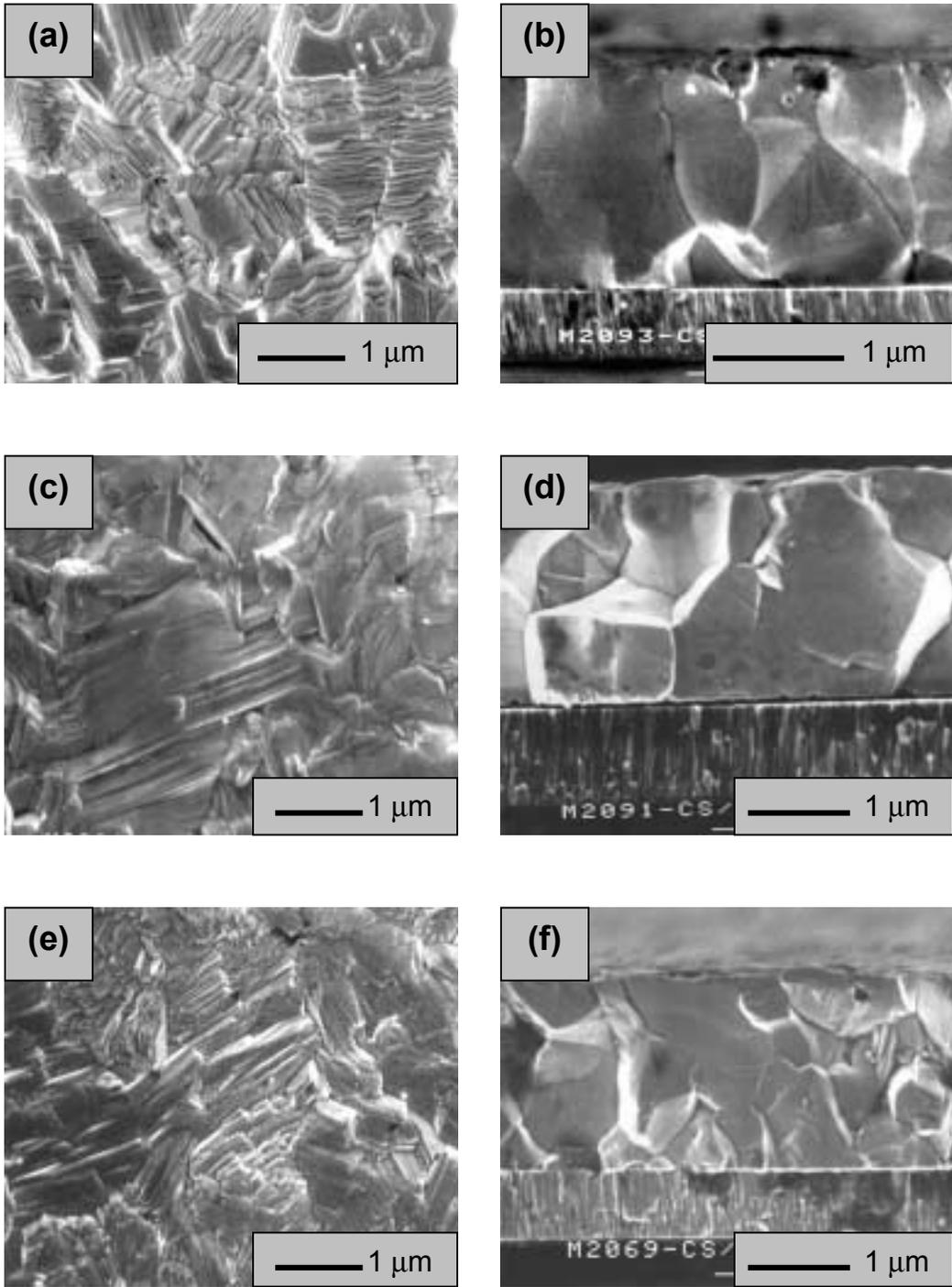
Fig. 5. SEM planar and cross-sectional views for CIGS films deposited on Mo sputtered films (a and b) at 0.8 mtorr, (c and d) at 5 mtorr, and (e and f) at 8 mtorr.
